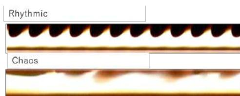
**Fig. 4 Cascade of bifurcation of the burning frame caused by the change of the height of the head of candle.**
